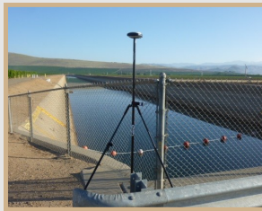
A GPS/GNSS receiver collecting data at an elevation monitoring station
